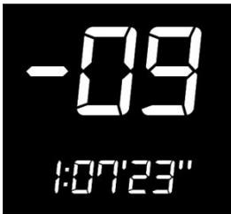
*In the upper portion, there are the allowed offences in countdown (the athlete is still allowed to make 9 more offences) and in the lower portion there is the chronometer, which also stores in the memory the exact moment of each offence or loss of contact*
