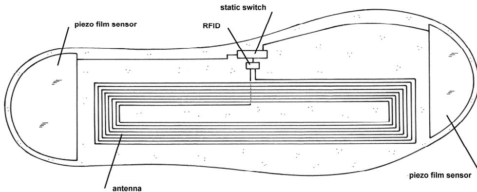
As can be noted, all the components are extremely thin and this makes possible that after the external sealed encapsulation of the insole, of silicone material or the like, the insole would be very thin, with a maximum thickness of 2-3mm.
